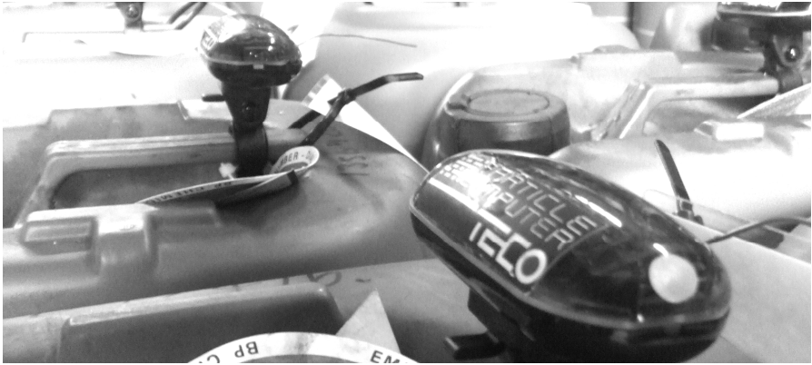
Fig. 1. Smart chemical drums equipped with sensor nodes
